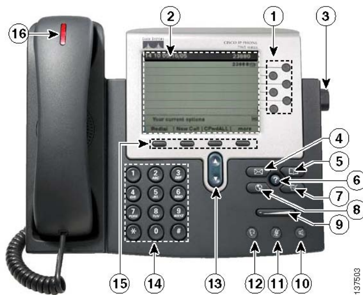
Figure 1 Cisco Unified IP Phone 7961G (the 7941G is identical but with only 2 line buttons)
